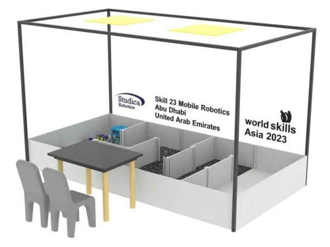
Two square LED Light Panels will be positioned over each Remote Clinic Court. The height of the frame will be set to ensure the lights are well above the head of a competitor standing in the court under these lights.
